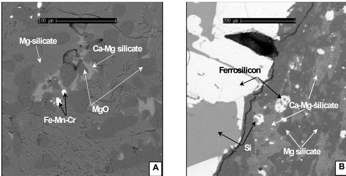
Figure 2: Back-scattered electron images of phases identified in the slags formed during Mg extraction from the magnesia-1.
