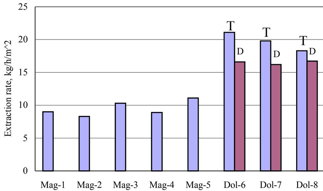
Figure 3. Average magnesium extraction rate (based on T: Tapped slag, D: Dig-out slag).
