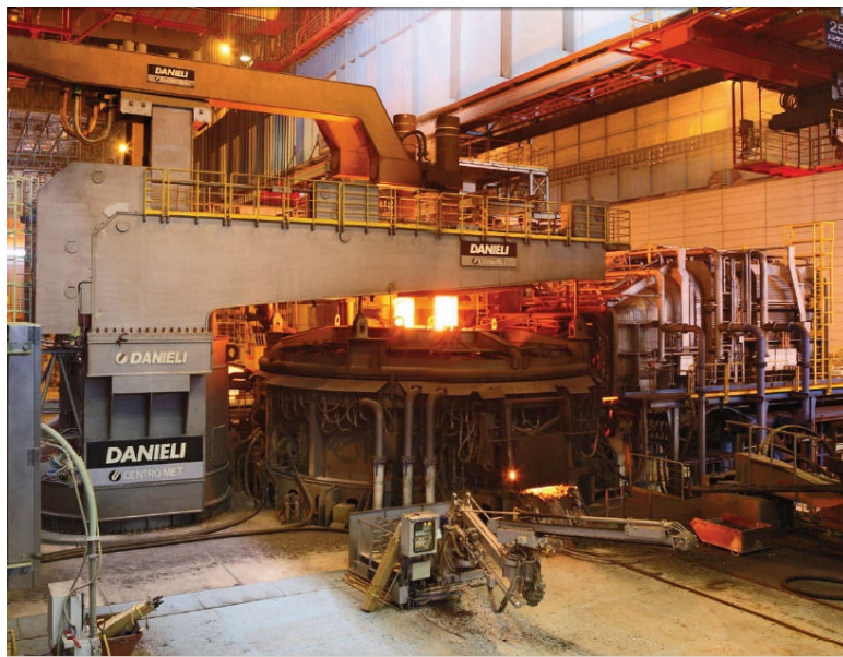
Figure 4. Tokyo Steel's 175 MW twin-cathode DC arc furnace
