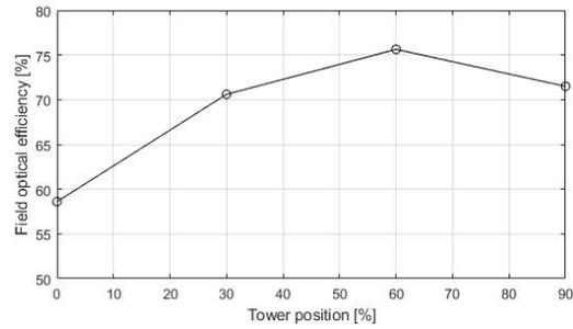
**Fig. 3** Tower position within field and resulting field optical efficiency.
