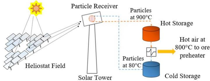
**Fig. 1** Concentrating solar thermal technologies.
