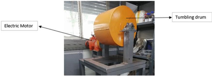
Fig. 2 A picture of a tumbling drum that will be used for the test
