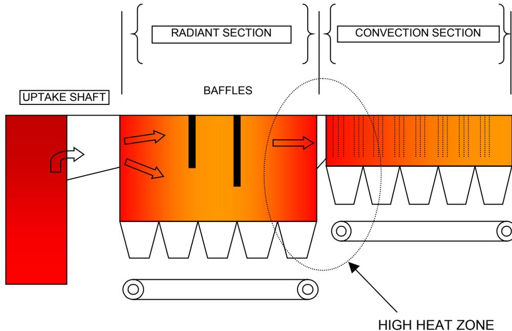
**Figure 19:** Planned waste heat boiler baffle installation
