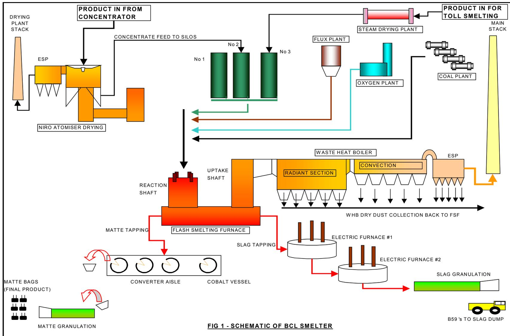
Figure 1: BCL Smelter Plant Flowsheet
