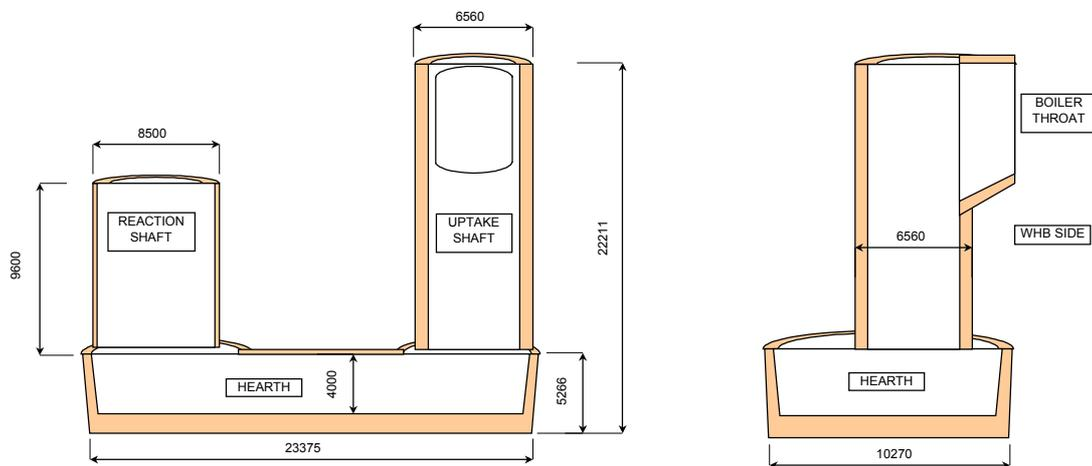
**Figure 2:** Dimensions of BCL Flash Smelting Furnace
